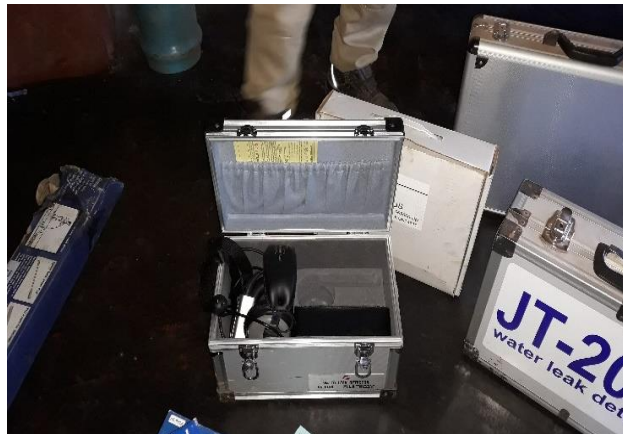
Figure 16: Leak detection equipment delivered to Shurugwi town council. Staff training on use of such equipment as well as overall safety and O&M training undertaken for technical staff across the towns under STWP.
