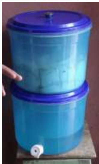
Domestic Defluoridation Unit
