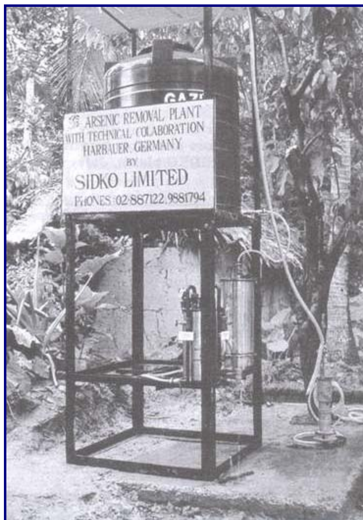
Water supply option: pilot arsenic removal plant (Ihteshamul Huq/DPHE)
